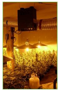
Carbon dioxide burner and propane tanks
